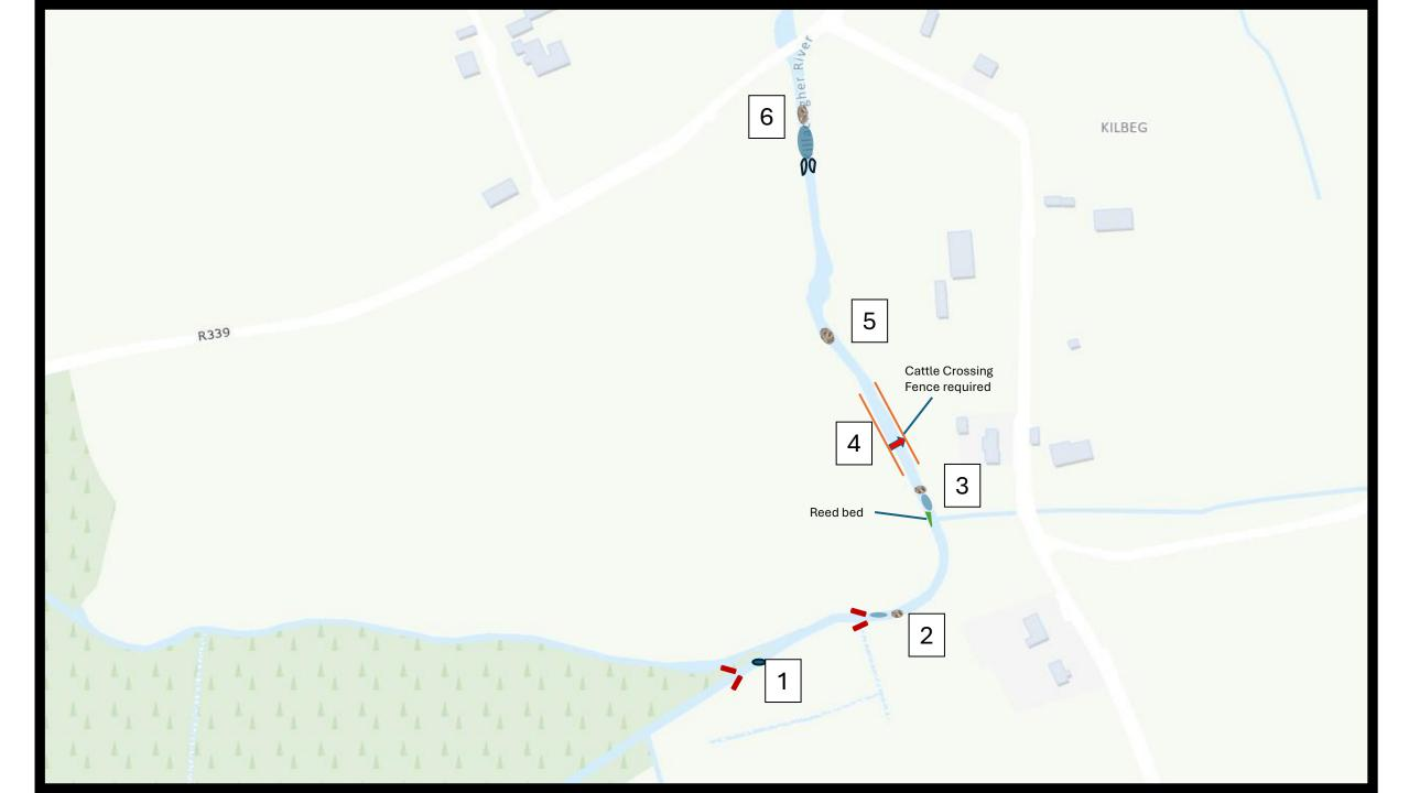
1. Use log structures to construct a paired deflector at location shown here.
