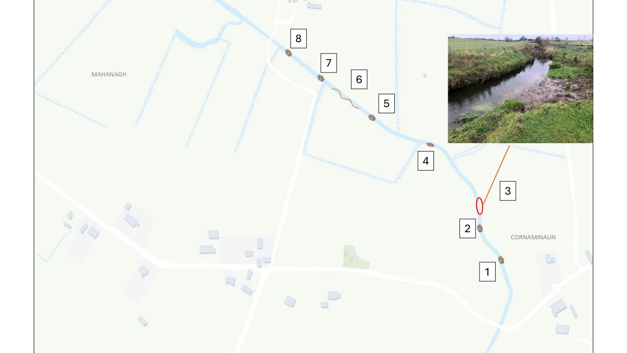
1. Ch. 23780 Place gravel bed (C. 3T) at gradient break.
